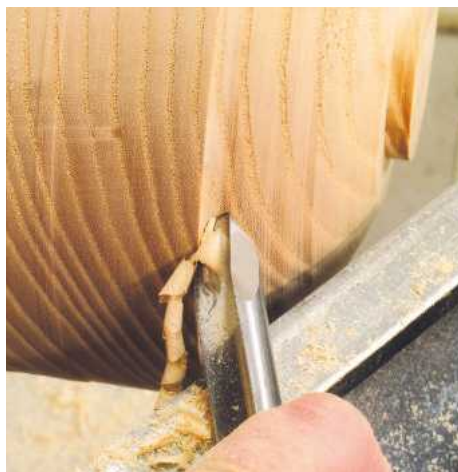
▲ Pic.5 This photo shows the cut perfectly: the wood is being cut and the shaving is rolling around the flute. Curly shavings are a good sign that the wood is being cut well
